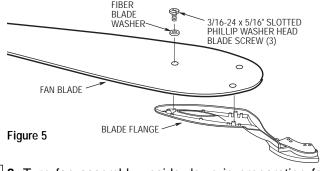
8. Turn fan assembly upside down in preparation for mounting fan blade assemblies.
